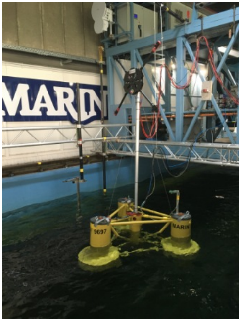
FIGURE 19. DEEPCWIND SEMISUBMERSIBLE WITH THE DRONE SYSTEM OF CENER
